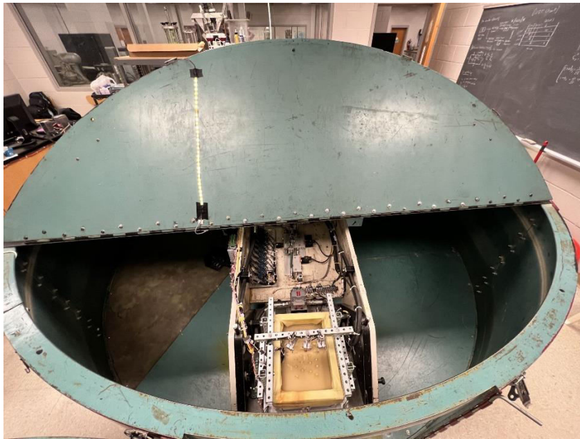
USC geotechnical centrifuge refurbished and installed at University of South Carolina
