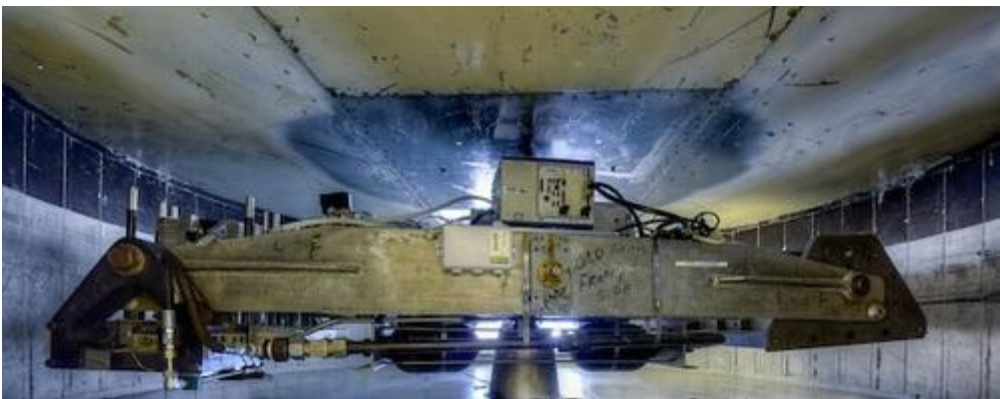
Geotechnical beam centrifuge refurbished and installed at UNH.
