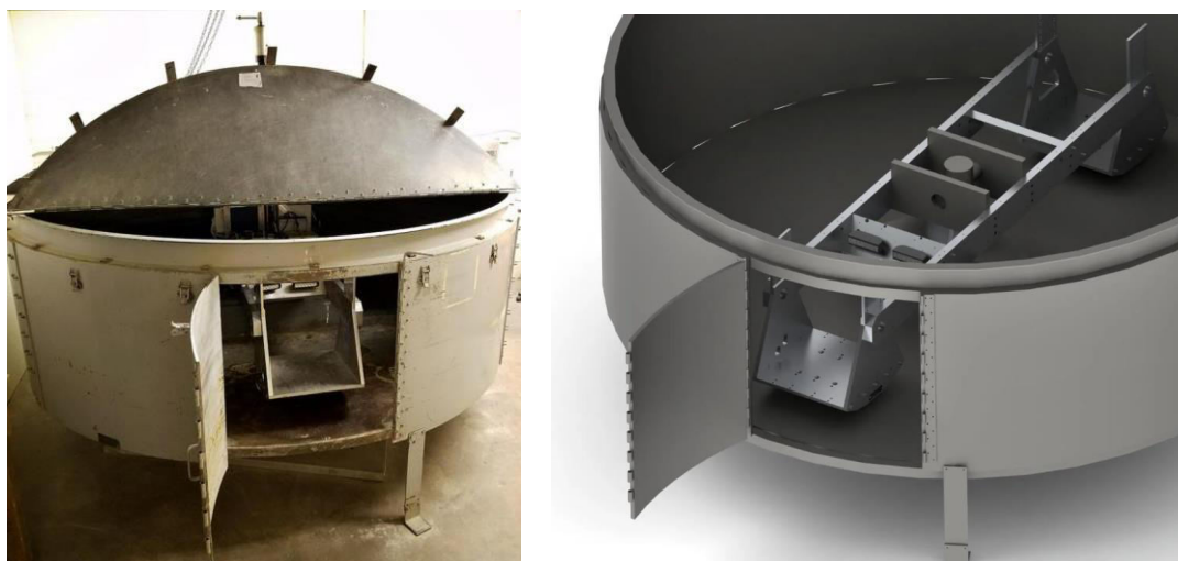
Photo and schematic of 15 g-ton centrifuge at CU Boulder
