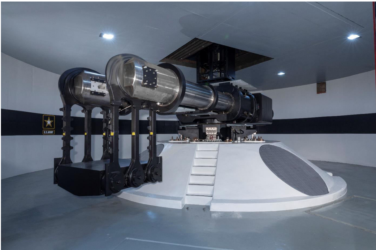
ERDC's geotechnical beam centrifuge recently refurbished (in 2022) and installed in Vicksburg, MS.
