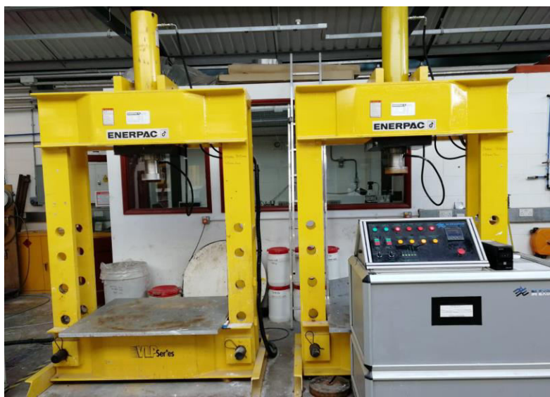
Hydraulic presses for clay sample consolidation
