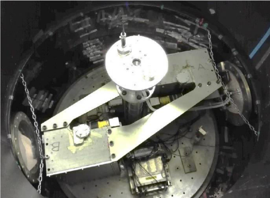
Broadbent geotechnical drum centrifuge with two cylindrical strongboxes installed.
