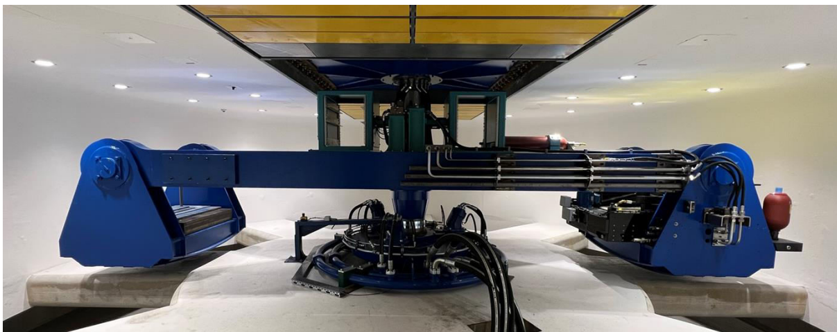
KRUPP geotechnical beam centrifuge refurbished and installed at ETH Zurich.
