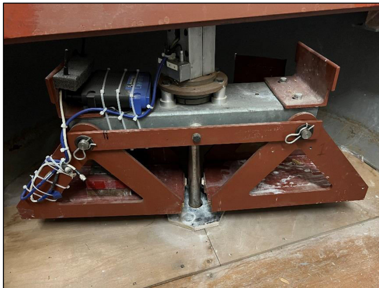
TU Delft 0.25 m-radius geotechnical centrifuge (TU Delft 2023)
