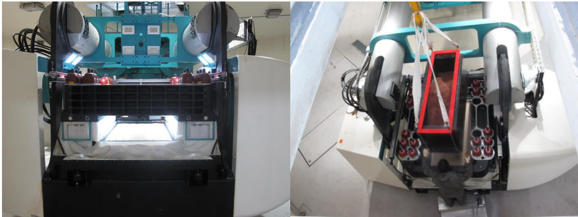
In-flight uniaxial earthquake simulator at K-water Research Institute
