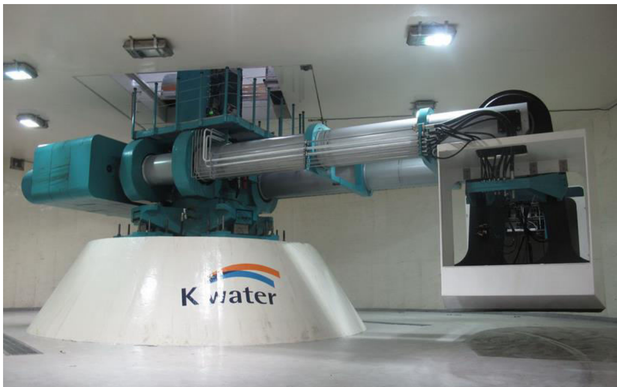
K-water geotechnical centrifuge
