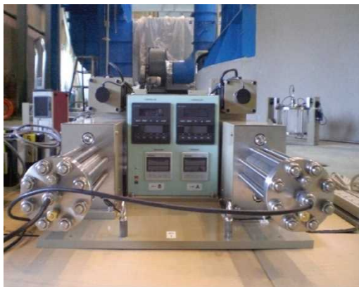
Water injection pressure pump
