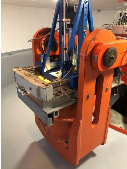
Load frame installed on the top of the cylindrical soil container. The frame is equipped with two actuators that apply controlled loading in the vertical and horizontal direction. Sketch of the setup after Truong et al. (2019)
