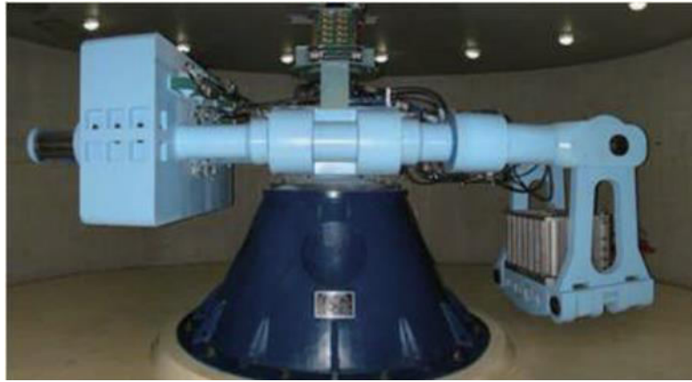
Single basket beam centrifuge developed and installed in Tongji.
