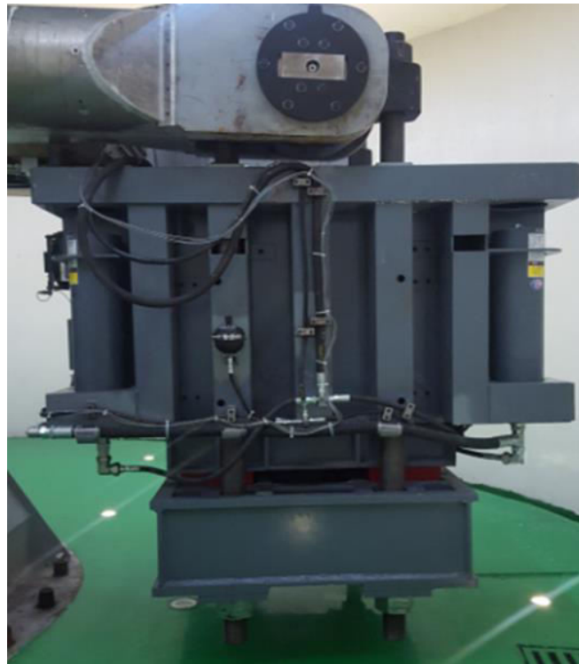
Schematic of the centrifuge earthquake simulator.
