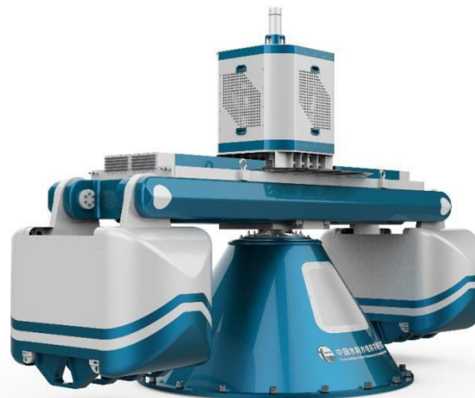
The IWHR 400 g-ton High-Speed Beam Centrifuge
