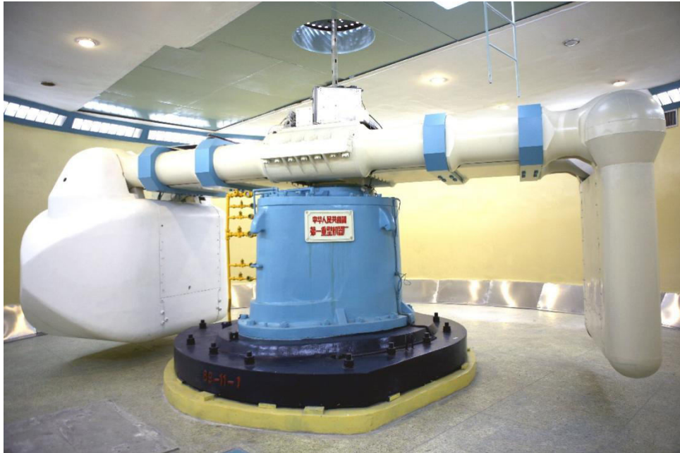
The IWHR 450 g-ton Beam Centrifuge
