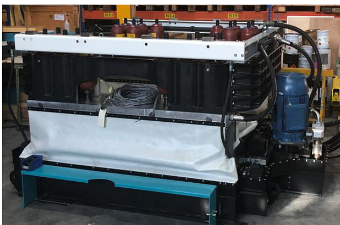
Actidyn on-board earthquake simulator
