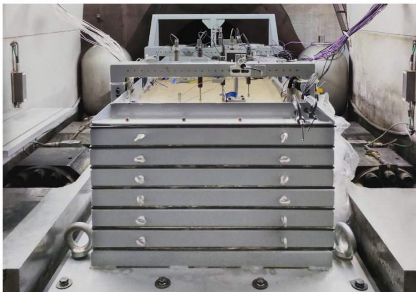
Fig3. A photo of the shaking table with a flexible shear beam container at IEM, CEA
