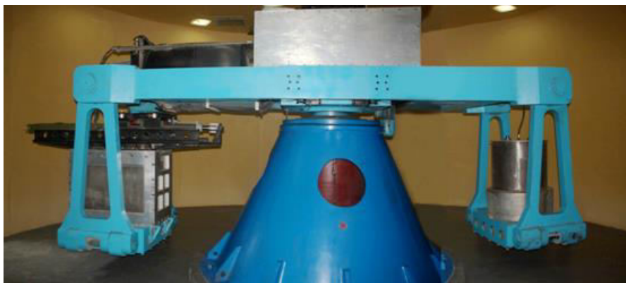
CKY-200 geotechnical centrifuge at Changjiang River Scientific Research Institute(2008, in use)
