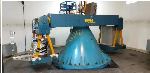
Wyle geotechnical centrifuge installed at UENF.
