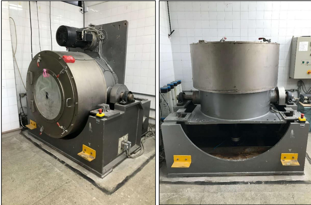
G-Max Scotland geotechnical drum centrifuge with two cylindrical strongboxes installed.
